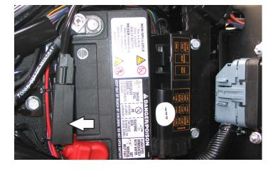
9 Remove the security module from the top of the battery.
