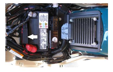
8 Remove the security module from the top of the battery. This unit slides to the right of the bike.
