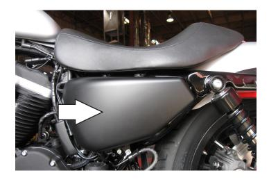
1 Remove the seat, left side cover, and battery.
