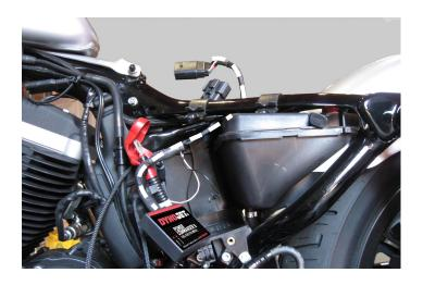
2 Route the large connectors of the PC6 harness underneath the frame tube to the area under the seat.
