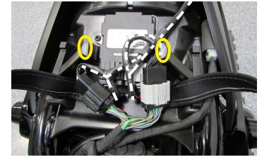
5 Plug the PC6 wiring harness in-line of the bike's ECM and both of the stock wiring harness connectors for the ECM.
