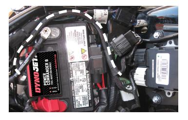
Install the PC6 in the cutout of the battery and route the harness to the right side of the battery.
