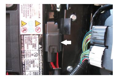
4 Position the fuse block so that it sits between the battery and frame.
