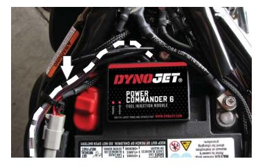
8 Using the supplied Velcro, secure the PC6 to the top of the battery.
