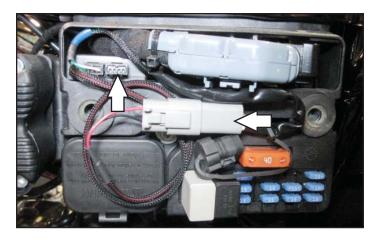
3 Using the supplied Velcro, install the Autotune module inside the electrical box next to the ECM.
