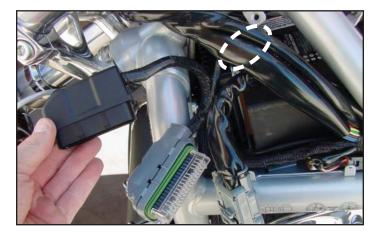
6 Plug the connectors from the PC6 wiring harness in-line of the stock wiring harness and the ECM.
