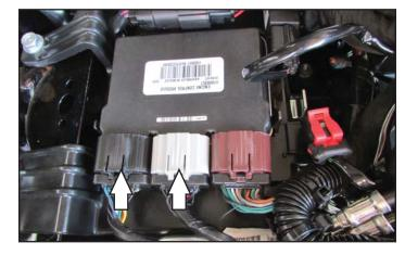
6 Plug the male connectors of the PC6 into the stock female connectors.
