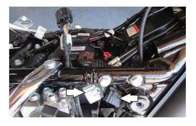
Route the stock ECM connectors that were disconnected in step 2 under the frame tube.
