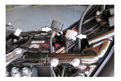
Route the female connectors of the PC6 behind the frame tube on the right side of the bike as shown. Slide the harness towards the rear of the bike.
