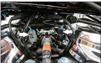
10 Plug the PC6 in-line of stock wiring harness and injectors.
