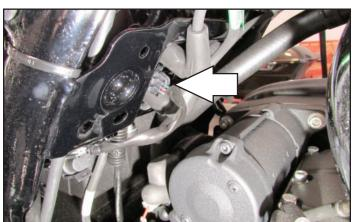
14 Connect the PC6 in-line of the stock wiring harness and ignition coil.
