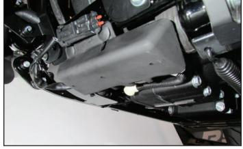
17 Unplug the stock Crank Position Sensor.
